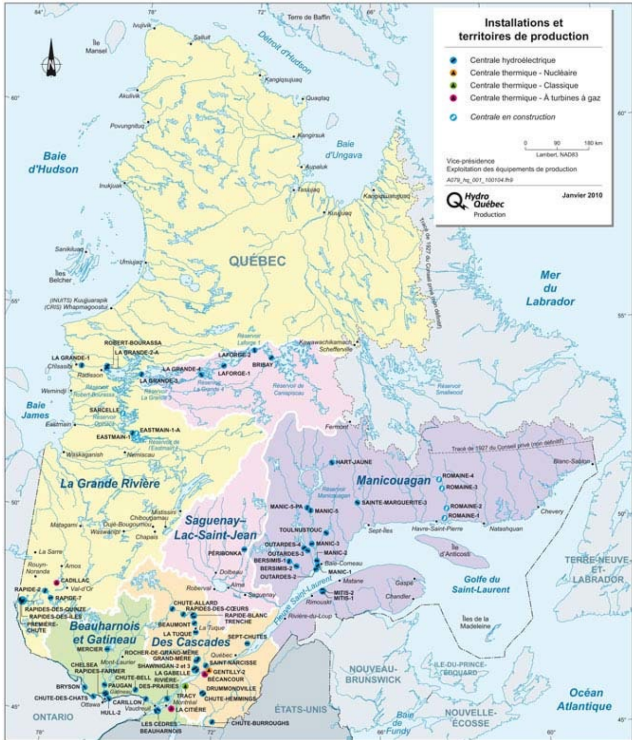
Figure 3: A 2010 map of the locations of major Hydro-Québec facilities. The map does not include substations and areas of neighboring connections. PHOTOGRAPHY BY RICHARD GERVAIS ET AL.
